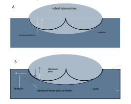
Figure 1 Theoretical model of hammock effect in wheelchair cushion. (A) The situation without a cushion cover, (B) The situation with a cushion cover. Friction from the cover develops causing additional tension along the cushion surface producing forces known as the hammock effect (lizaka et al. 2009)
