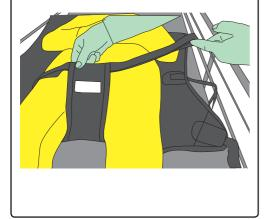
7 Attach the leg straps to the spreader bar followed by the shoulder straps. When starting the lift hold the slings bottom edge to prevent the sling from riding up.
