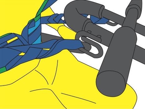
**6** Attach the lifting straps to the stand aid. The loop selection of each strap should be in accordance to a moving handling plan written by a competent person. Raise the stand aid until the straps start to take tension, stop the lift and ensure that all straps are attached correctly before completing the lift.
