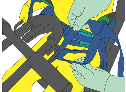
**7** The loop selection of each strap should be in accordance to a moving handling plan written by a competent person. Lifting straps can contain differing quantities of loops, the loop closest to the body of the sling will always be identified as number 1.
