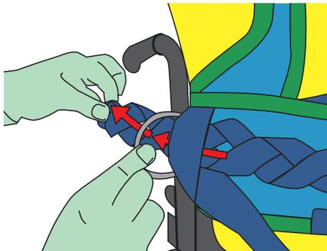
**5** Attach the crossover straps to the spreader bar.
